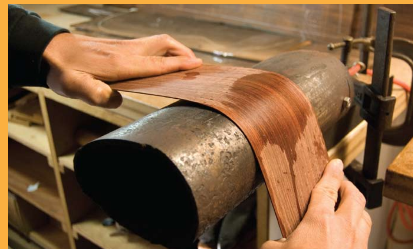
Wide, thin wood is wetted and bent over a hot pipe to make the sides of a guitar. Photo courtesy of Lewis Santer
