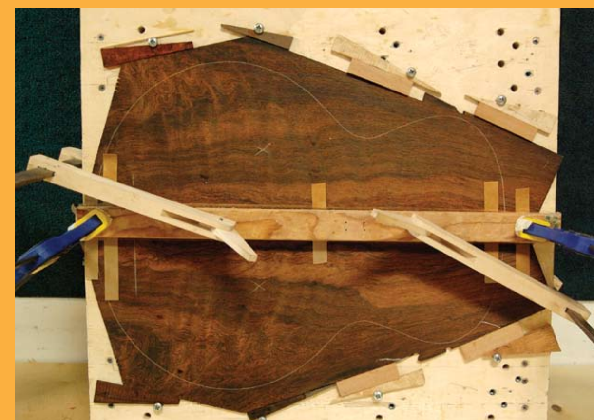
Bookmatched pieces of rough rosewood are glued together with a decorative center strip (here obscured by a long center clamp). White outline shows the final guitar shape. Photo courtesy of Lewis Santer
