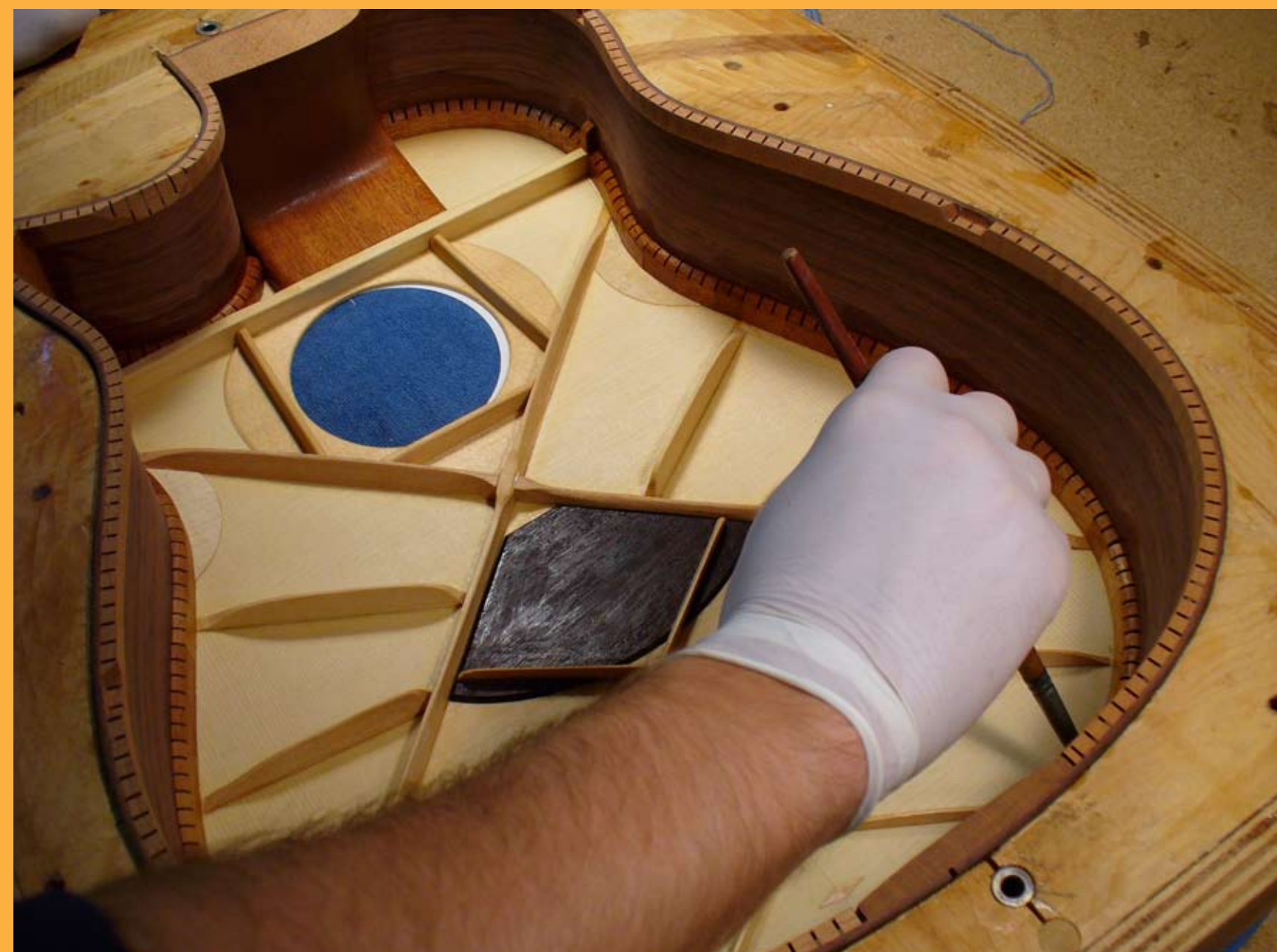
A top is glued onto its sides inside a guitar-shaped mold that holds everything in the correct shape. Before the back is glued on, the interior is brushed with shellac to seal it.
