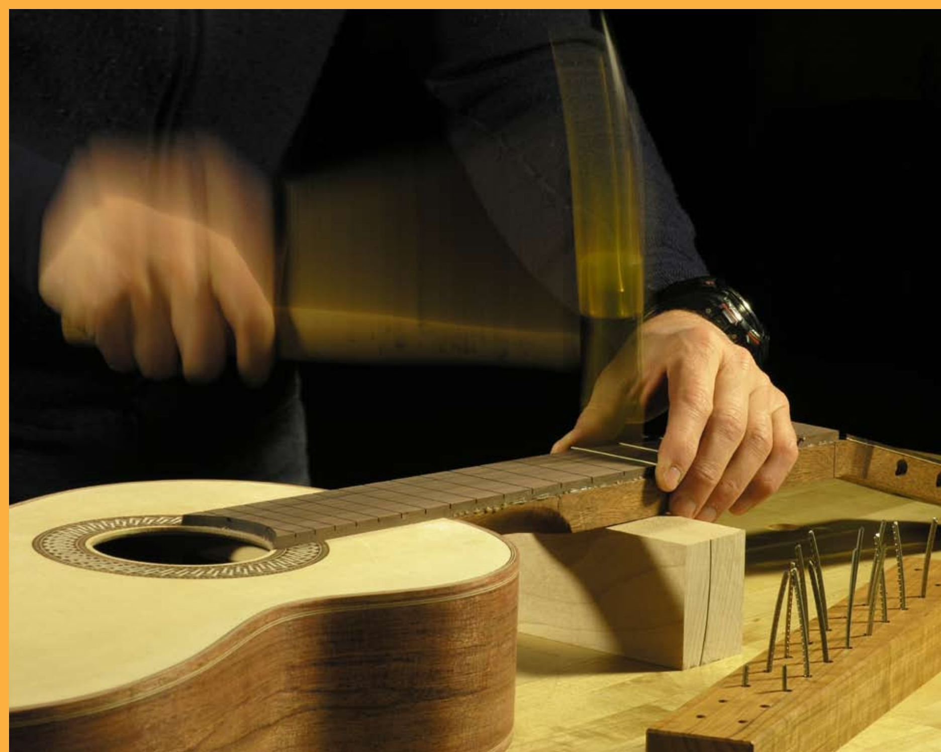
It may look a little dangerous, but careful hammering (and a well-supported neck) is the standard way to install frets into a fingerboard. Photo courtesy Erik Schmidt
