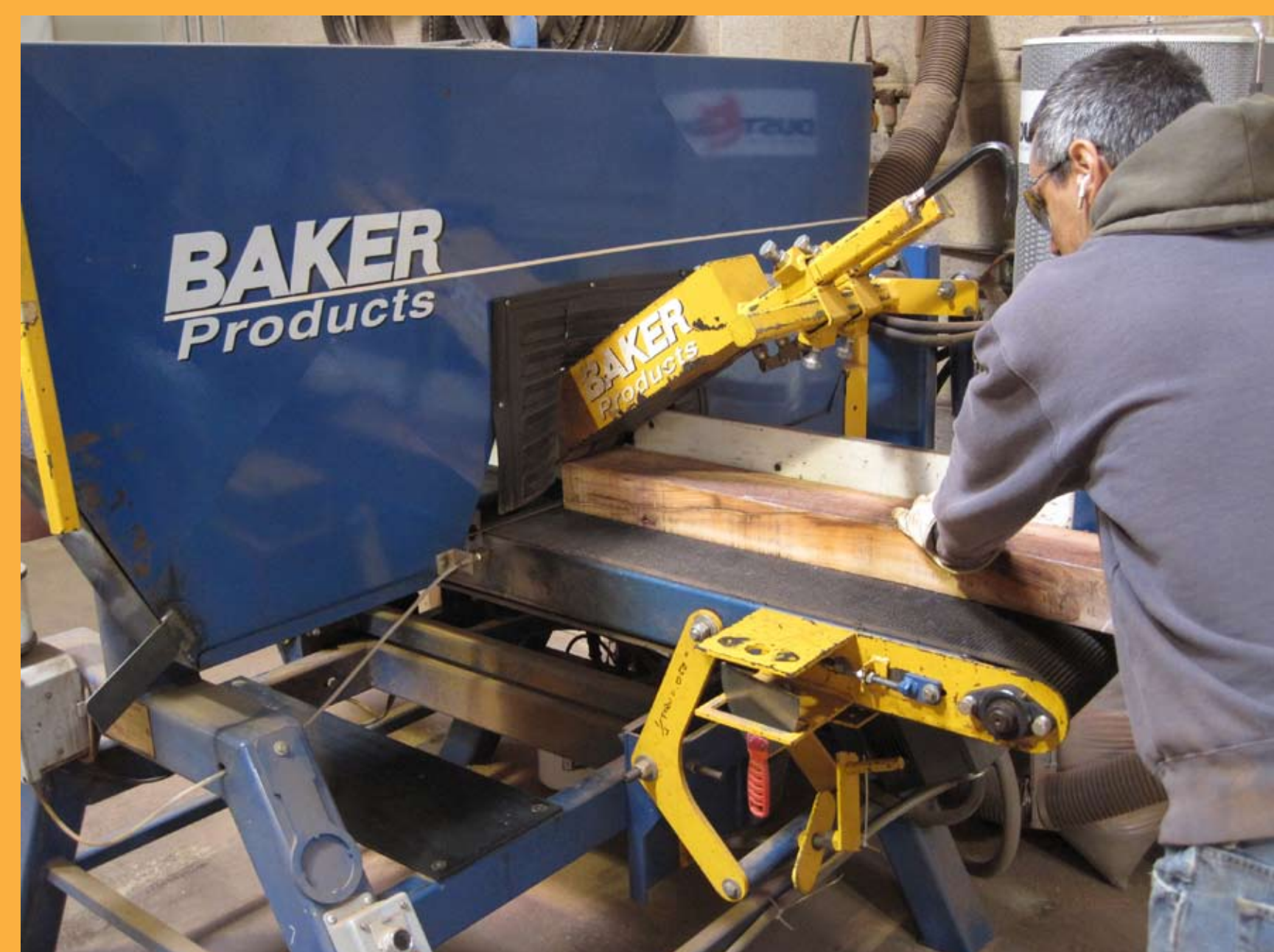
A quartersawn piece of instrument tonewood is sliced into sequential pieces for guitar sides. Photo courtesy of Todd Taggart, Allied Lutherie
