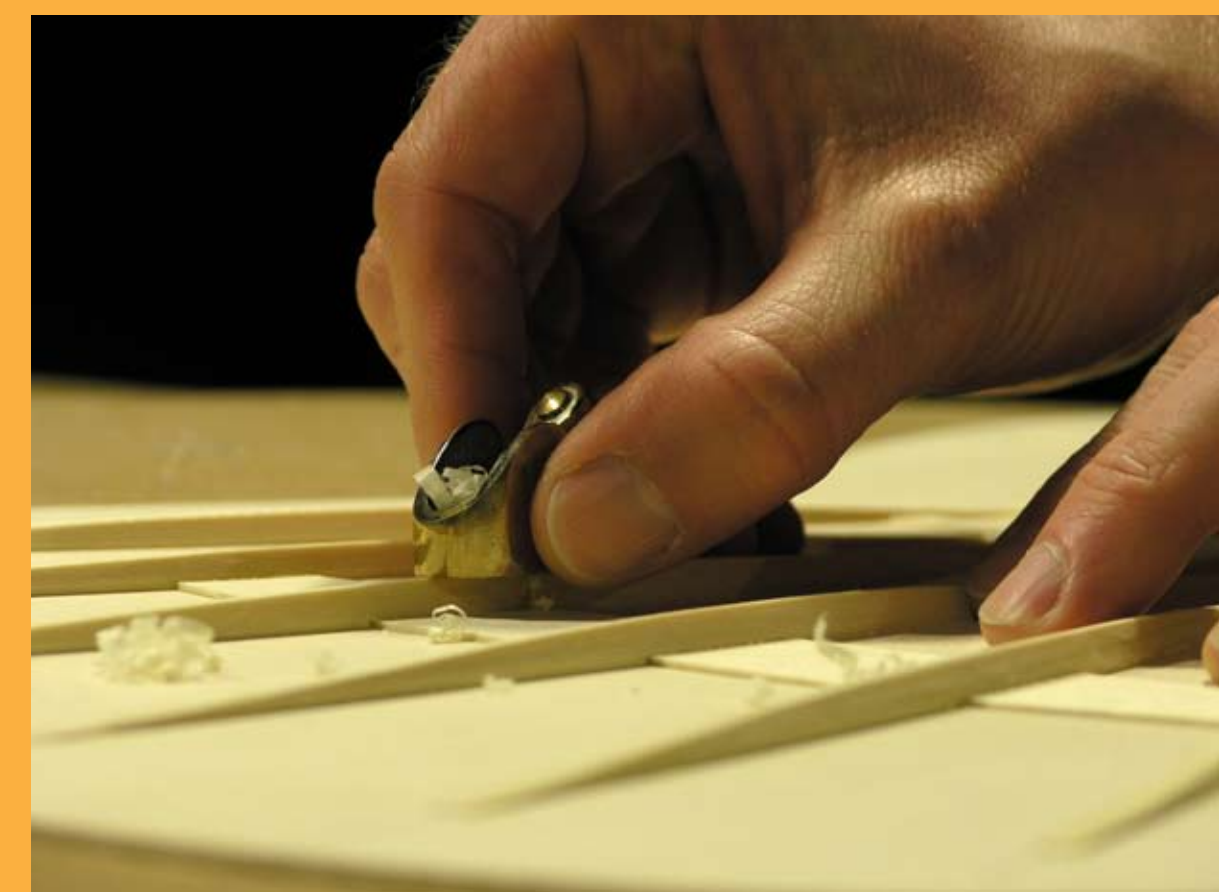
Stiffening braces are glued to tops and backs. Here, top bracing is being hand planed to its final shape. Photo courtesy Erik Schmidt
