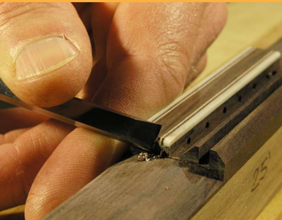
Finishing up the final details on a bridge before it is glued onto your new handmade guitar! Photo courtesy Erik Schmidt
